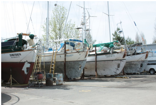
Ladd's Marina, Stockton, March 2012— Tortuga, Worldwind, Pelican, and Amablè receive the hull fairing modification.
