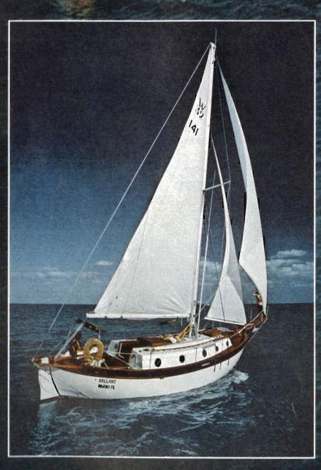
Left: Pictured here is possibly the ultimate in cruising sailboats—the Westsail 32, a lovely wide-beamed, double-hulled 32-footer that sleeps four (six in a pinch) and includes such practical ocean-going features as a low freeboard, a small self-boiling cockpit and a full keel. Inside, the Westsail is a shipshape sanctum of rich woodwork. Fully equipped for the high seas, the Westsail runs about \$60,000.
